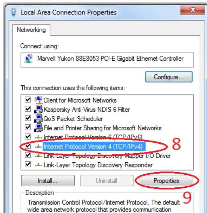
Zatim čekirajte opcije **Obtain an IP address automatically** (10) i **Obtain DNS server address automatically** (11) i potvrdite na **OK** (12).
